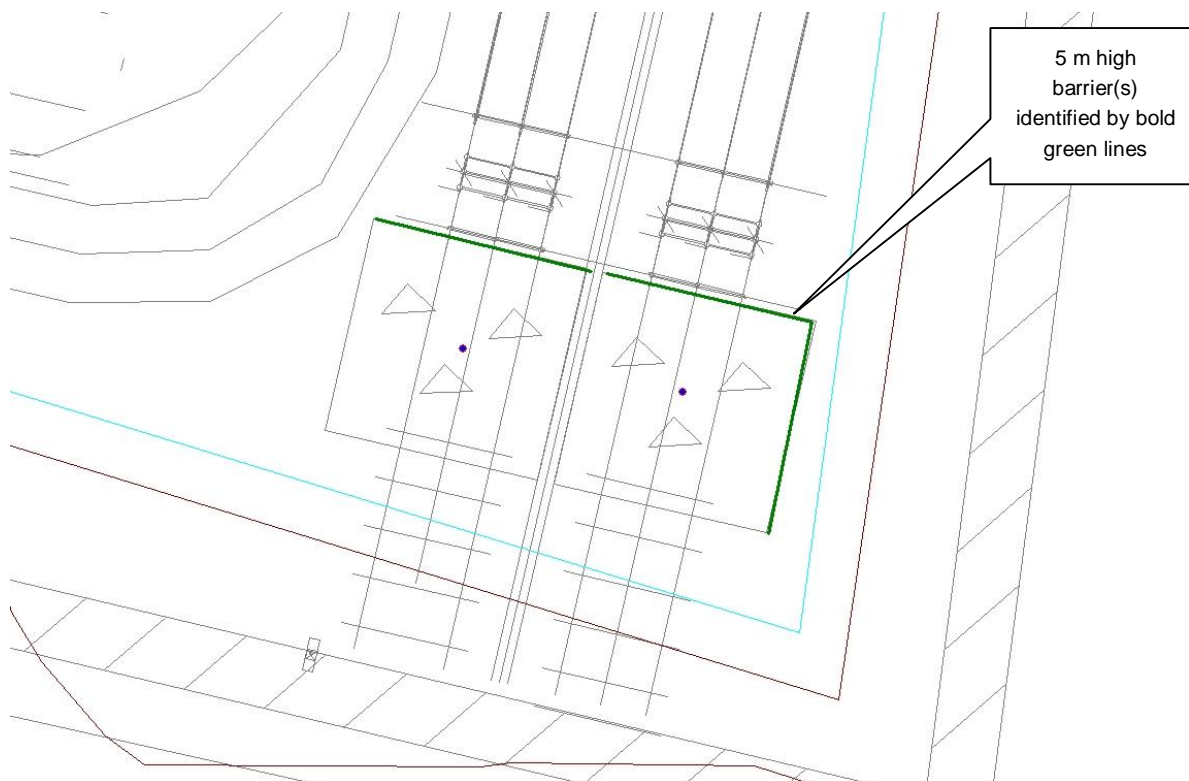
Figure 3 – Location of 5 m barrier around reactors
