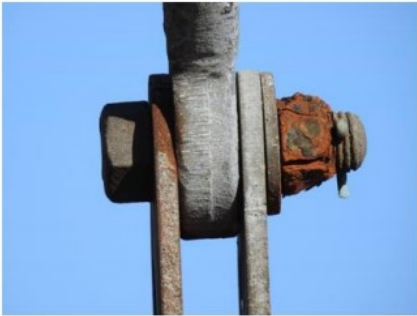
Figure 2-3 Corroded conductor and earthwire fittings
