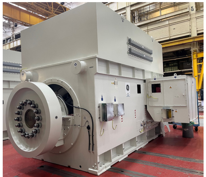
Synchronous condensers like this one will be installed to maintain power flow.
