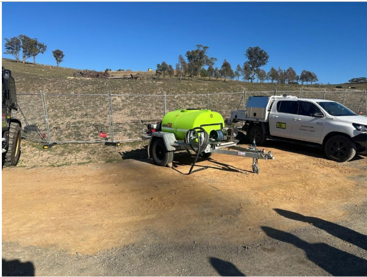
Photo 43: Trailer mounted fire fighting unit
