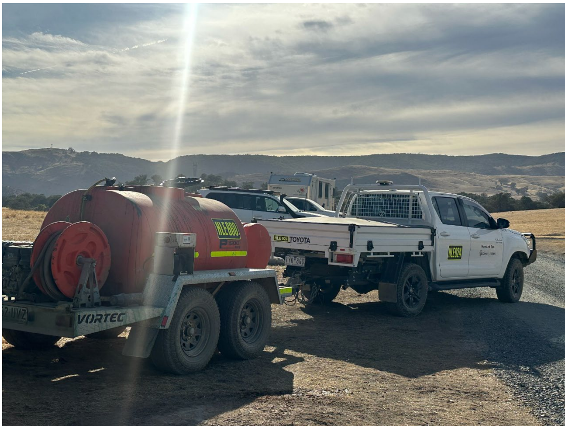
Photo 67: Trailer mounted fire fighting unit
