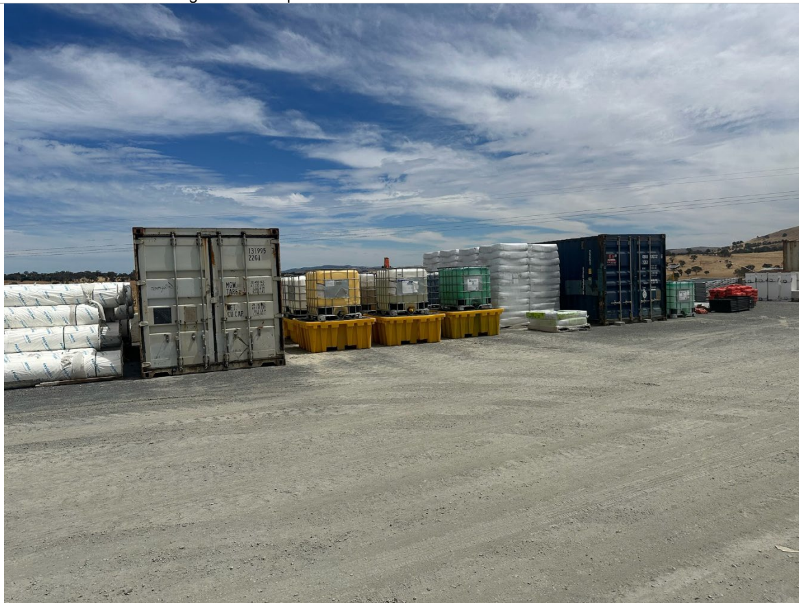
Photo 24: Chemicals stored in mobile bunding
