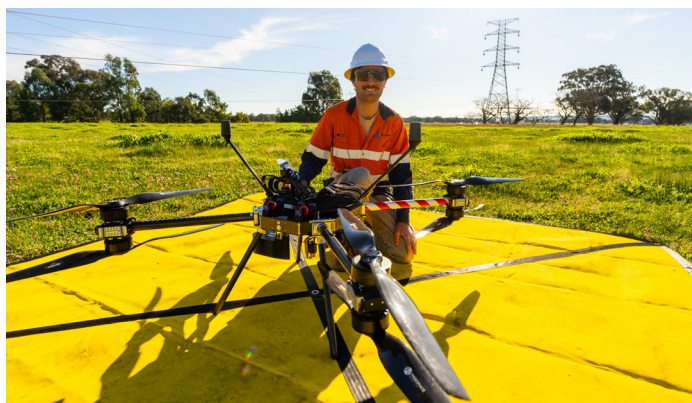
Pilot Phillip Phoebe prepares his drone for another stringing flight.
