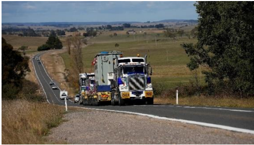
Shunt reactor on route to Bannaby substation.
