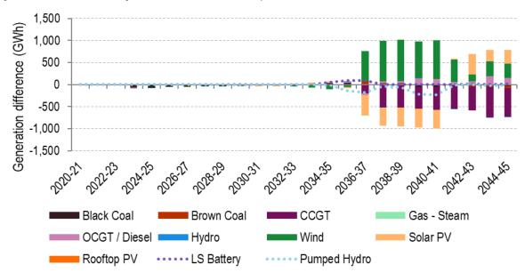
Figure 21: Difference in NEM generation forecast between Option 4 and Base Case
