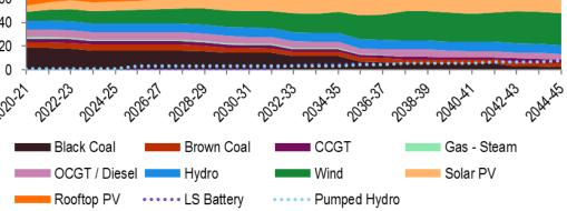
Figure 2: NEM generation mix forecast for the Base Case in the Central scenario  $^{11}$
