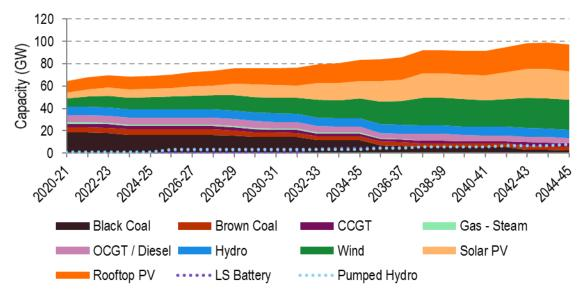
Figure 8: NEM capacity mix forecast for the Base Case
