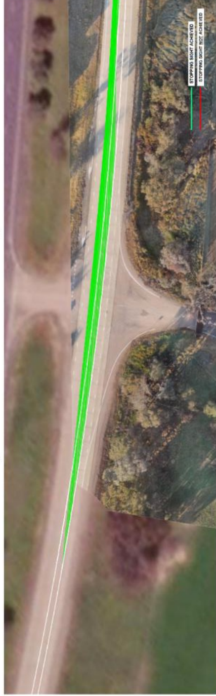
STOPPING SIGHT DISTANCE - NORTHBOUND CARRIAGEWAY
