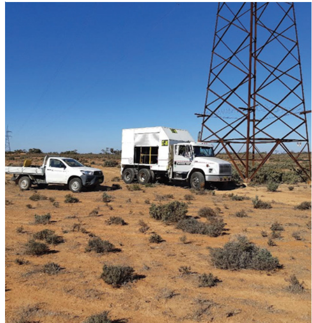
CPT rig on site with support vehicle
