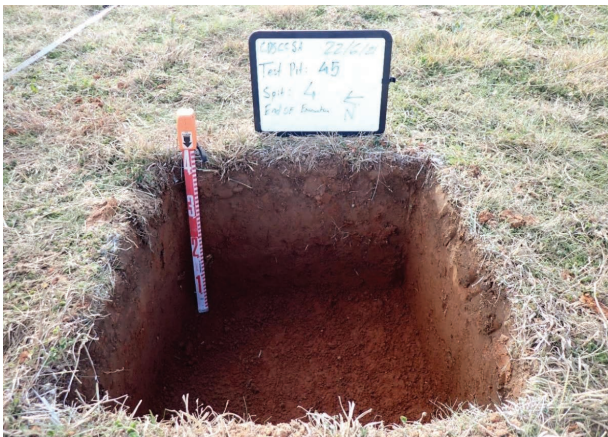
Excavated pit (0.5 m x 0.5 m pit size)
