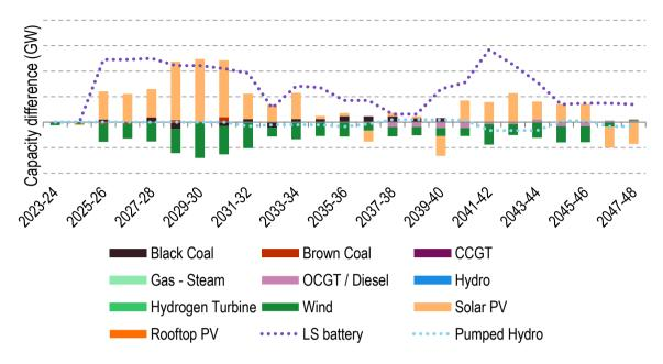
Figure 26: Difference in NEM generation forecast between Option 1A(2) and Base Case in the Step Change scenario (including forecast generation of Option 1A(2))
