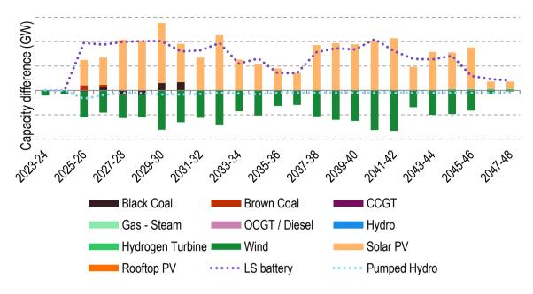
Figure 23: Difference in NEM generation forecast between Option 1A(4) and Base Case in the Hydrogen Superpower scenario (including forecast generation of Option 1A(4))
