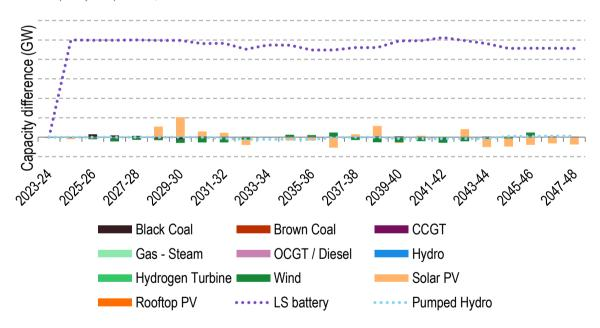
Figure 38:Difference in NEM generation forecast between Option 5G and Base Case in the Step Change scenario (including forecast generation of Option 5G)
