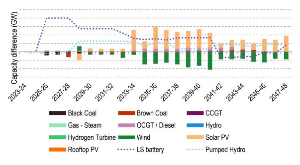
Figure 20: Difference in NEM generation forecast between Option 1A(4) and Base Case in the Progressive Change scenario (including forecast generation of Option 1A(4))
