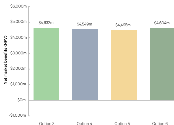
Figure 8.13: Net market benefits sensitivity – Alignment with NSW Roadmap projects and assumed diesel generation constraints, Step Change scenario ($2024/25)
