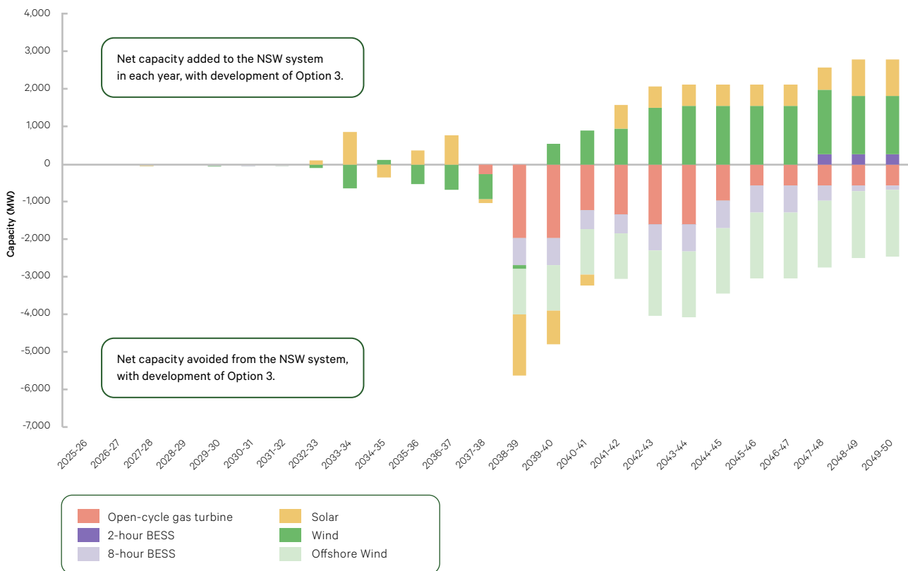
Figure 8.2: Impact of developing Option 3 on the optimal generation mix in NSW vs counterfactual base case, Step Change scenario
