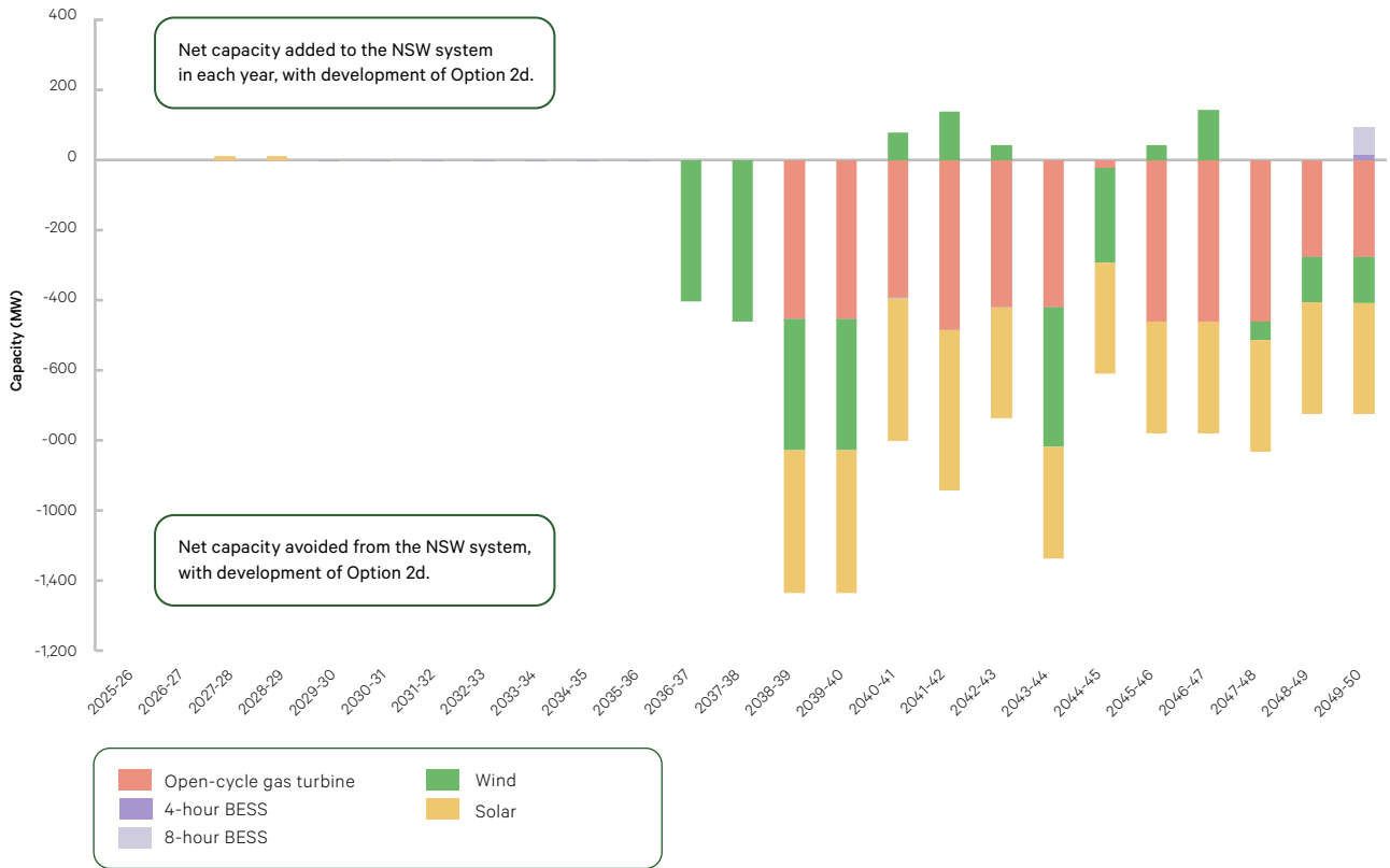
Figure 8.8: Impact of developing Option 2d on the optimal generation mix in NSW vs counterfactual base case, Slower Growth scenario
