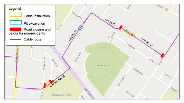
A cable drum behind a large truck will bring the cable to site at Centennial Street. The drum and truck are around 4.5 metres wide when parked and six metres wide when in use, and will arrive before the morning peak time and turn off its engine until 7am. It will leave after cable installation has ended.
