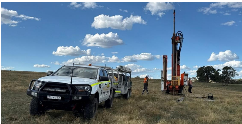
A geotechnical inspection using a borehole drill to collect soil samples near Biala
