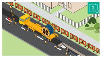
At each joint bay, sections of cable are pulled through the underground pipes. This takes around two weeks.
