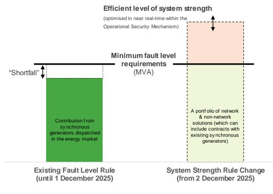
System strength can broadly be described as the ability of the power system to maintain and control the voltage waveform at any given location in the power system, both during steady state operation and following a disturbance
