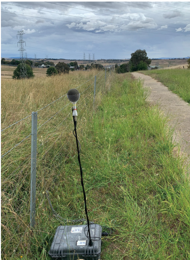
Pictured: Noise logger used to measure background noise levels in an area.
