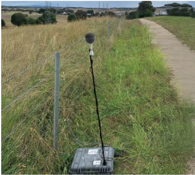
Figure 4: Noise logger used to measure background noise levels.
