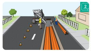
Trenching involves digging a trench around three metres wide and installing pipes to house the cables. Work takes around two weeks near each property.
