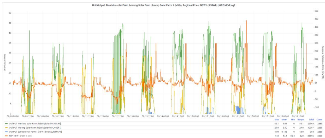
Figure 3. The generation profiles of Molong, Suntop 1, and Manildra solar farms from 09/09/2022 to 18/09/2022 5
