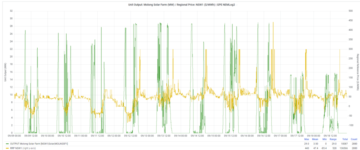
Figure 4. The generation profiles of Molong solar farm from 09/09/2022 to 18/09/2022 6
