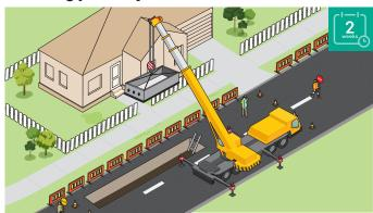
Joint bays are installed roughly every 900m along the cable route. Work takes around two weeks at each location.
