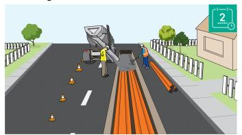
Trenching involves digging a trench around three metres wide and installing pipes to house the cables. Work takes around two weeks near each property.
