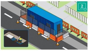
Sections of cable are joined together at the joint bay. This takes a further two weeks.
