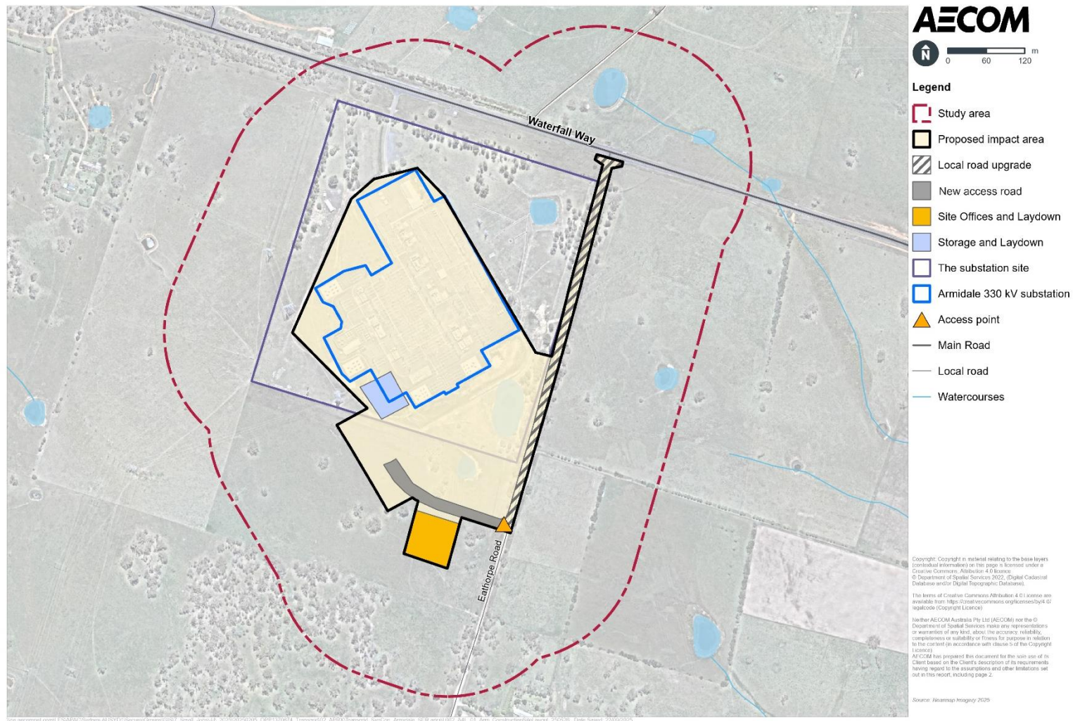
Figure 1-3 Proposed impact area and indicative construction site layout
