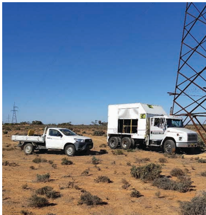
CPT rig on site with support vehicle
